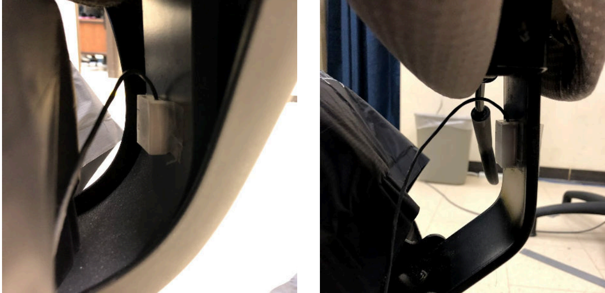
Figure 1: Location of the accelerometer on the rigid arm of the seat pan for both the CoreChair (left) and the control chair (right) respectively.
