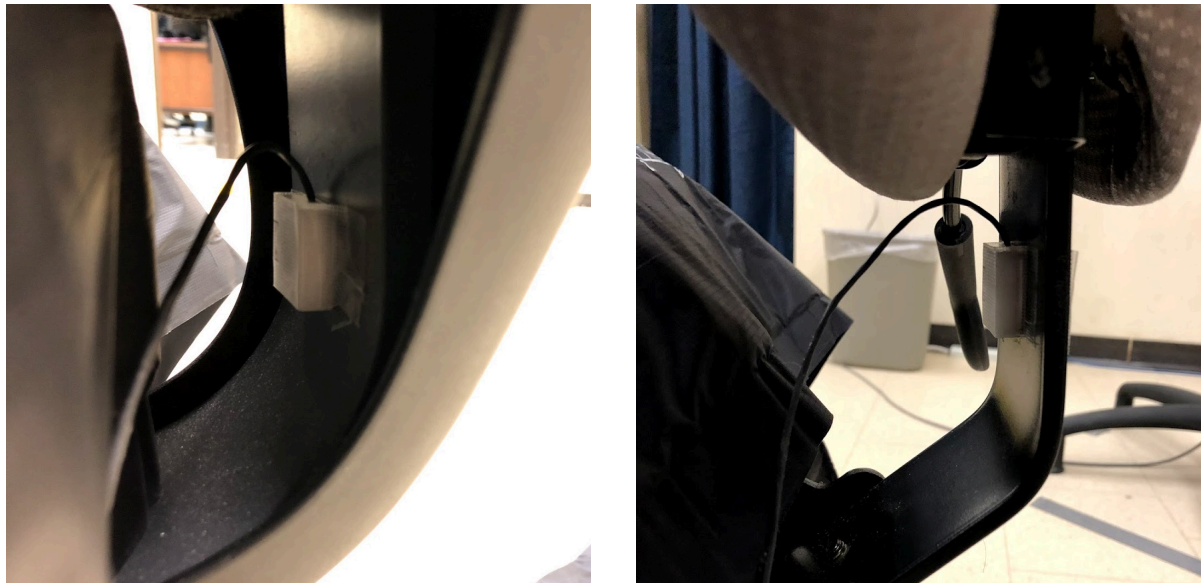
Figure 5: Location of the accelerometer on the rigid arm of the seat pan for both the CoreChair (left) and the control chair (right) respectively.
